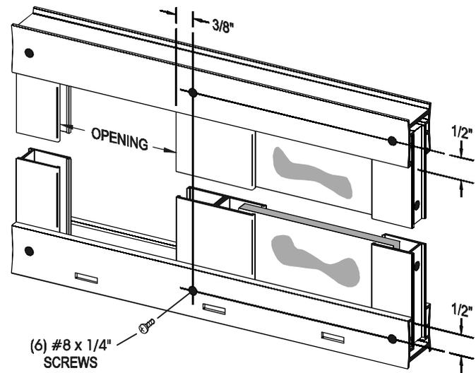
**CAUTION:** To prevent damage to the glass panel, drill the holes on the door side of the post.
