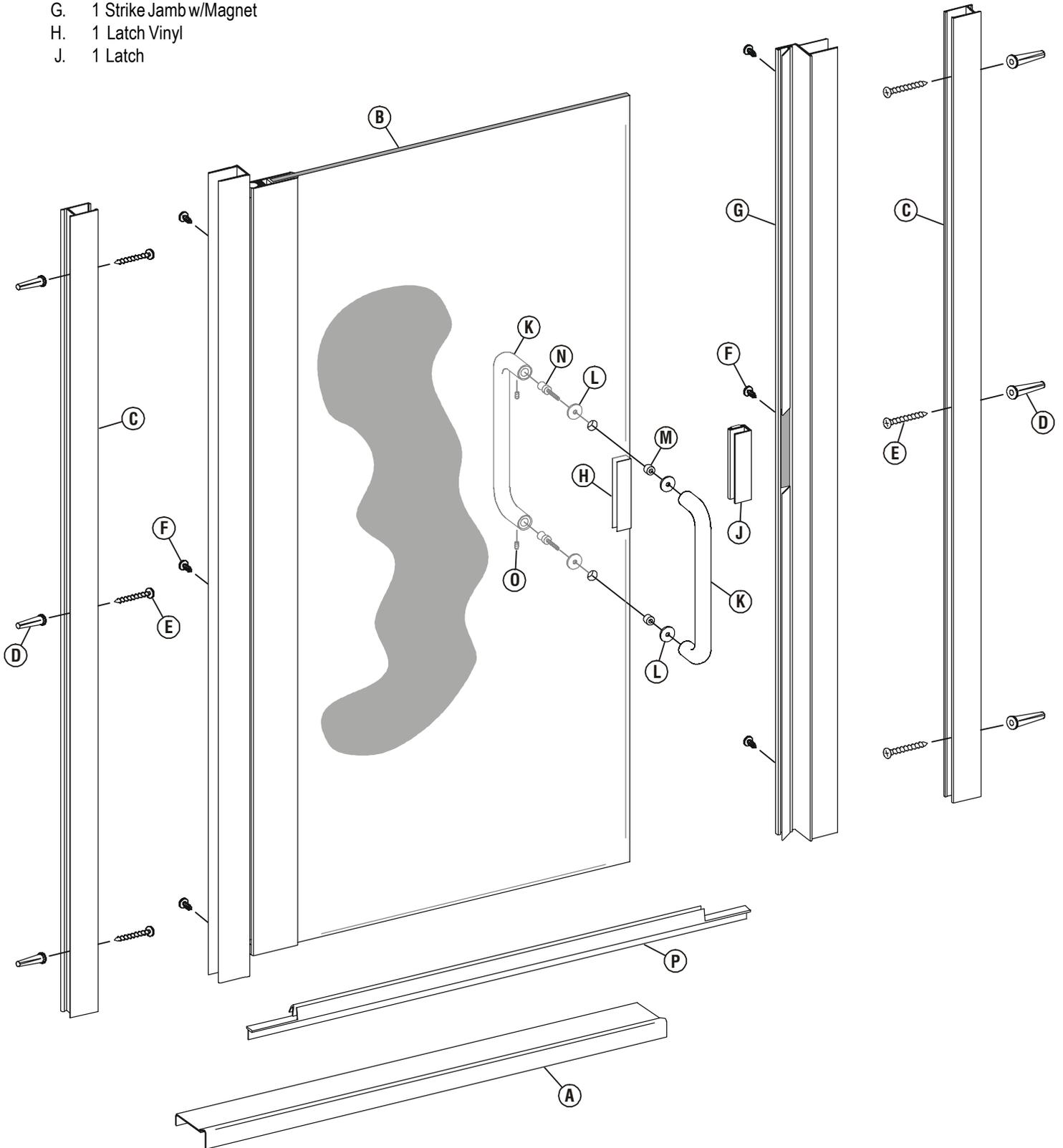
**1** The Alumax 300cv Continuous Hinge Shower Door is completely reversible and may be installed hinge-left or hinge-right. Refer to the illustration to determine the correct position for your installation. For maximum waterproofing, the hinge jamb should always be opposite the shower head. These instructions depict a hinge-left installation.
