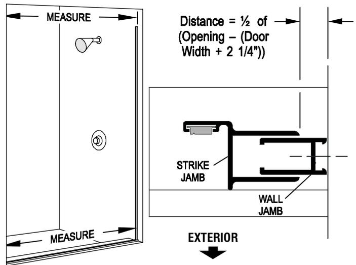
**5** Inside the shower enclosure, drill two 1/8" holes thru the strike jamb [G] and into the wall jamb [C] 3/8" to 3/4" from the wall and approximately 1" vertically from each end of the strike jamb. Drill a third hole centered between the first two, then enlarge the three outer holes with a 3/16" drill for clearance on the self-tapping screws. Attach the strike jamb permanently with three #6 x 3/8" pan head screws [F].
