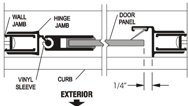
**7** Inside the shower enclosure, drill two 1/8" holes thru the hinge jamb and into the wall jamb [C] 3/8" to 3/4" from the wall and approximately 1" vertically from each end of the hinge jamb. Drill a third hole centered between the first two, then enlarge the three outer holes with a 3/16" drill for clearance on the self-tapping screws. Attach the door panel assembly permanently with three #6 x 3/8" pan head screws [F].
